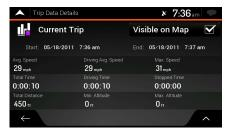
By tapping on the Trip Data Details screen, you can view the trip on the map, export track logs, and check the elevation and speed profiles.
