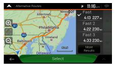
If there are suitable alternatives calculated with the route planning method that is selected in Route preferences (page 70), they are shown on top of the list. Routes with other route planning methods are shown at the bottom of the list.
